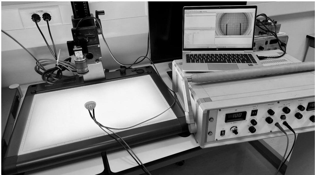
**Figure 2:** Experimental setup showing the camera rig and the agarose sample under treatment in a petri dish (diameter of 34 mm) with a custom-made cover/electrode holding guide, pulse generator, and laptop computer for controlling the camera and recording video data.
